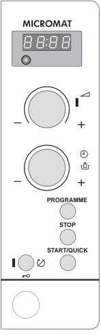
1. Plug the appliance into the mains. The display starts to flash «AEG» and then «OO:OO». The dots between the digits blink rapidly.
